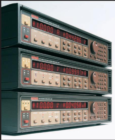
The 236, 237, and 238 Source-Measure Units (SMU) are fully programmable instruments, capable of sourcing and measuring voltage or current simultaneously. These systems are really four instruments in one: voltage source, current source, voltage measure, and current measure.
