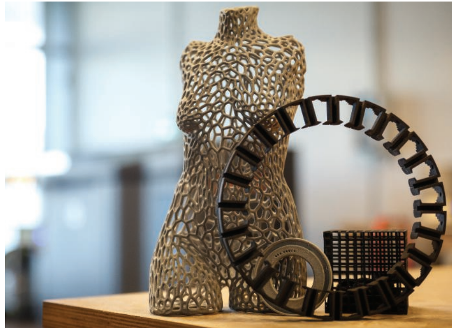
Below: Weerg's HP 3D printers can generate plastic parts competitively versus injection moulding up to quantities of 110,000
