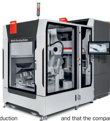
The new Mobile Bending Robot attached to a Bystronic Xpert 40 press brake
