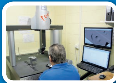
Frictec employs both tactile and camera-based inspection on its 640 by 900 by 500 mm Axiom Too from Aberlink
