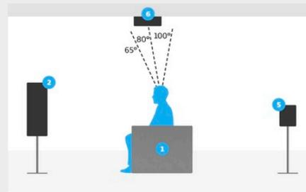
Overhead speaker placement detail for 5.1.2 setup
