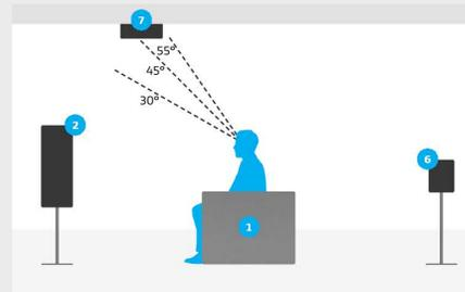
Overhead speaker placement detail for 7.1.6 hybrid setup
