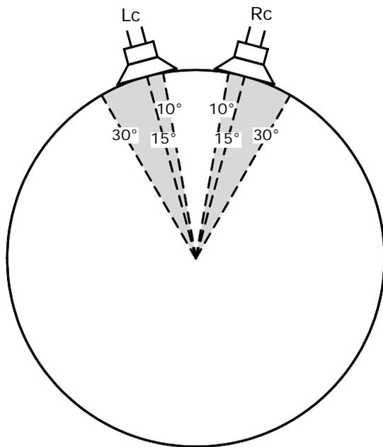
Figure 27: Left center and right center speaker placement.
