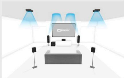
Perspective detail for 5.1.4 hybrid setup
