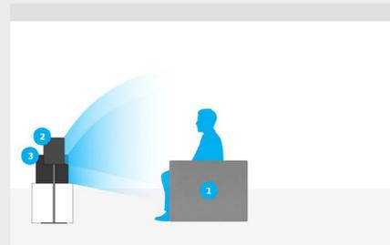
Virtual speaker placement: detail for 3.1 setup
