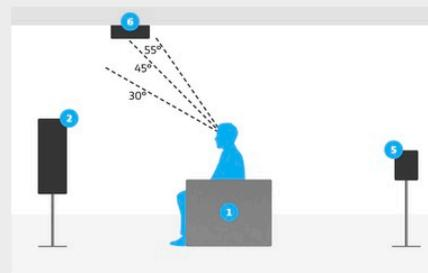
Overhead speaker placement detail for 5.1.4 hybrid setup
