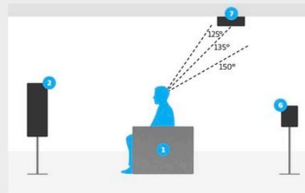
Overhead speaker placement detail for 7.1.4 hybrid setup
