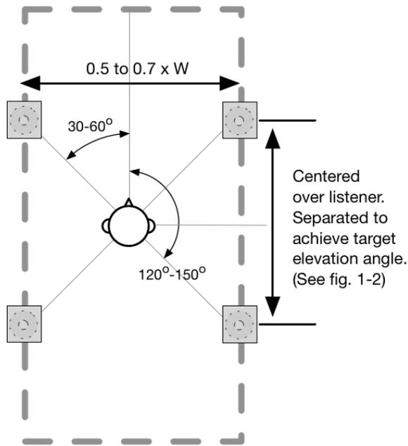
Figure 4: Top view, height (overhead) speaker positioning.
