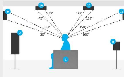
Overhead speaker placement detail for 11.1.8 setup
