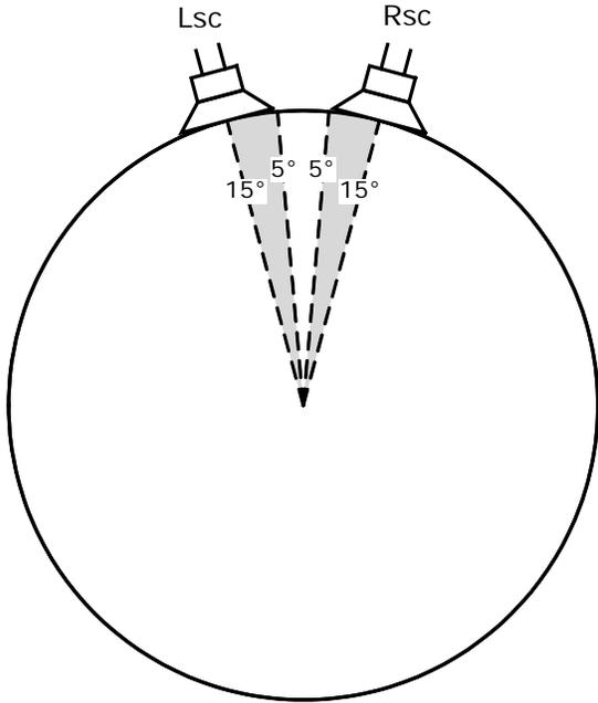
Figure 28: Left screen and right screen speaker placement.
