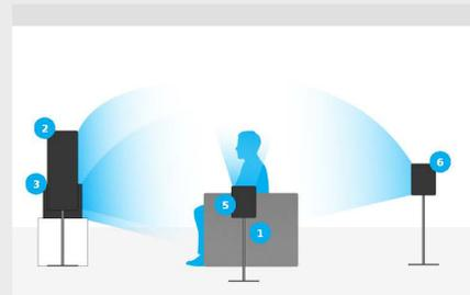
Virtual speaker placement: detail for 7.1 setup
