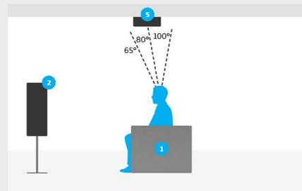
Overhead speaker placement detail for 3.1.2 setup
