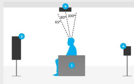
Overhead speaker placement detail for 4.1.2 setup
